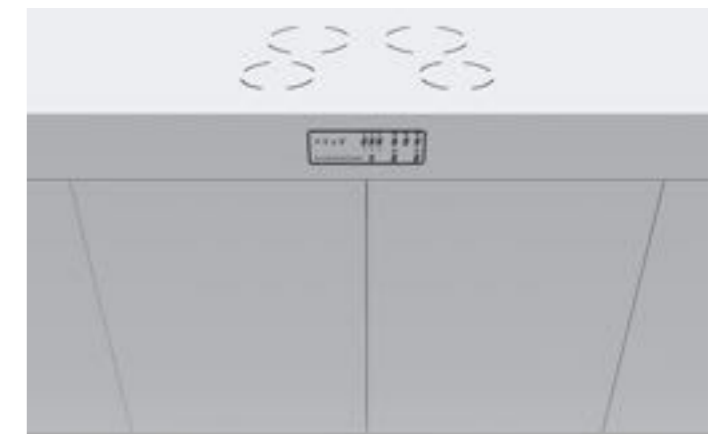
in the worktop and folded front panel, folding min. 145 mm, see picture
